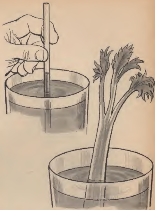
Capillary action causes the water to rise in the straw above the water level in the glass, and makes the coloured water rise through the stalk of celery.
